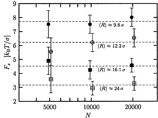
FIG. 5. Tensile force  $F_z$  as a function of system size for systems of different ratio  $L_z / N$ : (●) 0.01, (○) 0.008, (■) 0.006, and (□) 0.004. The corresponding average radius  $\langle R \rangle$  is also indicated. A slight horizontal offset is included to improve visibility of the error bars.
