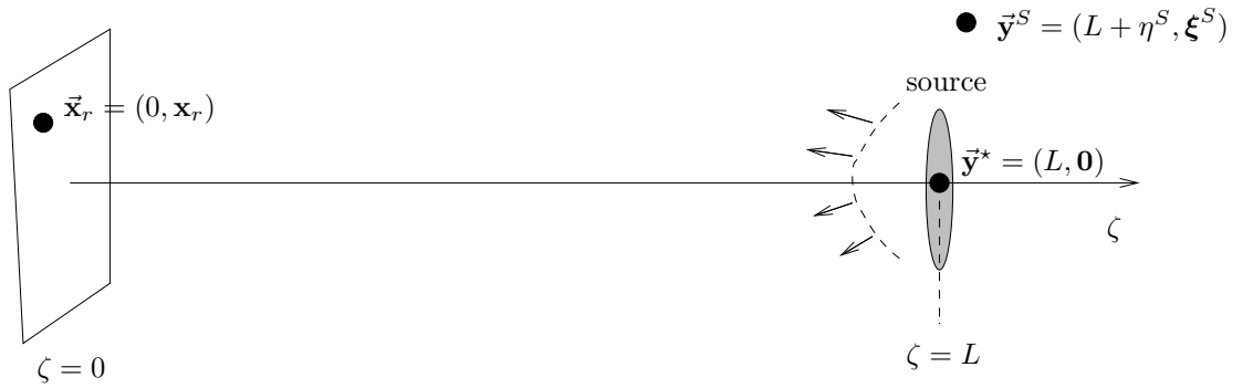
Figure 1: Setup for imaging a distributed source with a planar array of transducers
