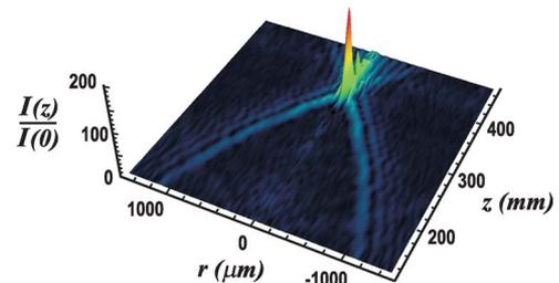
Fig. 3. (Color online) Radially averaged intensity as a function of the propagation distance. Intensity values are normalized to the peak intensity at  $z = 0$ .
