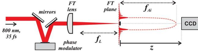
Fig. 1. (Color online) Experimental setup. FT, Fourier transform;  $f_L$ , FT lens focal length;  $f_{Ai}$ , effective focal length of the Airy ring.
