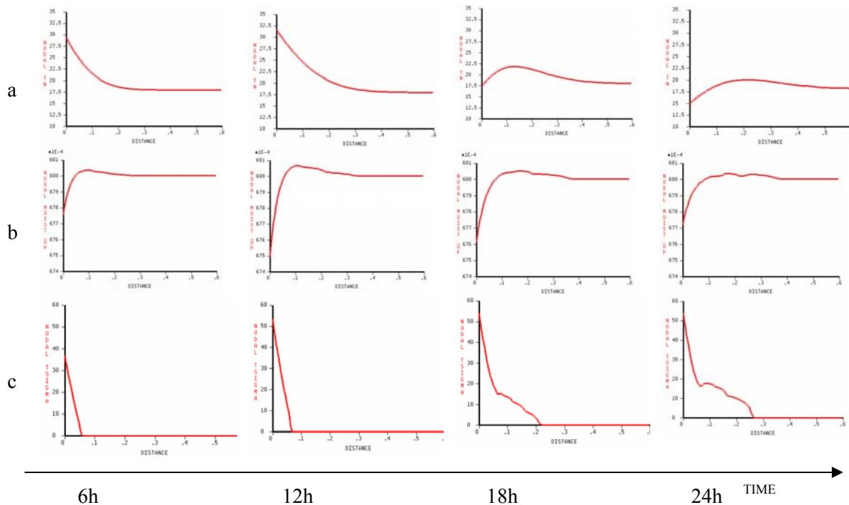
Figure 5: Variation along the simulated strip (bag-air interface at 0 m, bag centre at 0.6 m) of (a) temperature (in °C), (b) solids moisture content (in %), (c) caking strength (in Pa) at various times during a 24-hour cycle.
