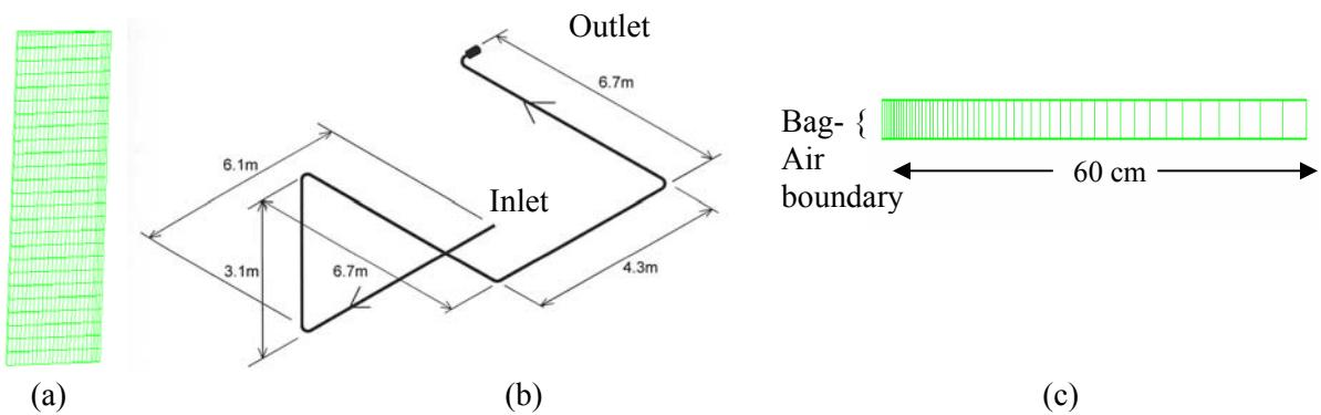
Figure 1: (a) Applied geometry and mesh for the core flow flat-bottomed bin (segregation), (b) The pneumatic conveying system (degradation), (c) Applied mesh for simulated bag strip (caking).
