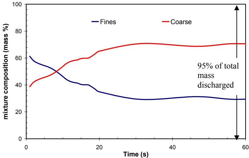
Figure 3: Temporal segregation profile of the individual mixture components during core flow discharge.
