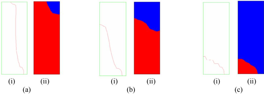
Figure 2: Development of (i) flow / no-flow boundary, (ii) interface between material (red) and air (blue) at times (a) 2s, (b) 30 s and (c) 60 s. The channel above the orifice is maintained filled until the creation of the final stagnant region at the material angle of repose.
