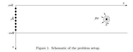
We consider acoustic wave propagation in a two dimensional inhomogeneous waveguide with planar horizontal boundaries as the one depicted in Figure 1. The acoustic pressure field  $p(t, \vec{x}) = p(t, x, z)$  is governed by the scalar wave equation
